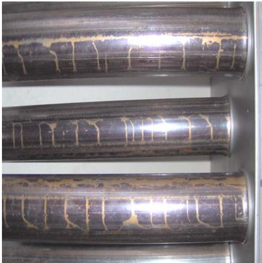
Figure 7: Dark and Streaky Surfaces of Laser Welded and Annealed Tubing
