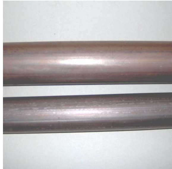
Figure 8: Varying Degrees of Surface Staining/Coloring in Laser Welded and Annealed Tubing
