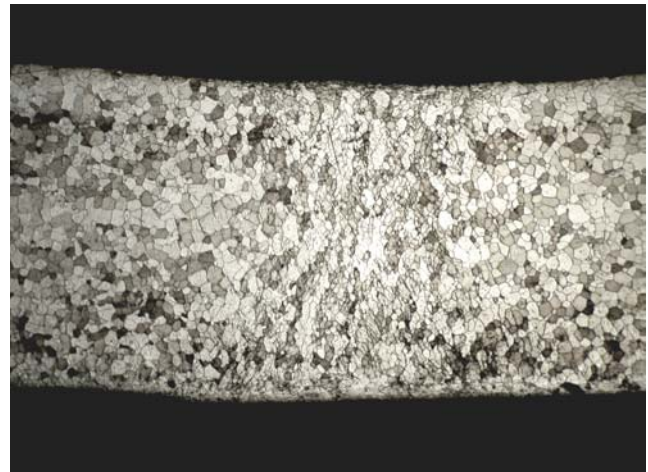
Figure 10: Typical UHFSS 409 SS Tube Weld Zone/HAZ
