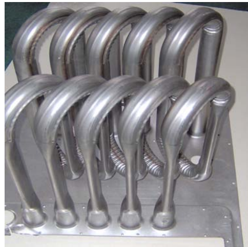
Figure 1: Tubular Heat Exchanger
